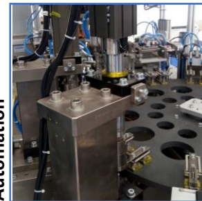
Bearing Pressing Automation
